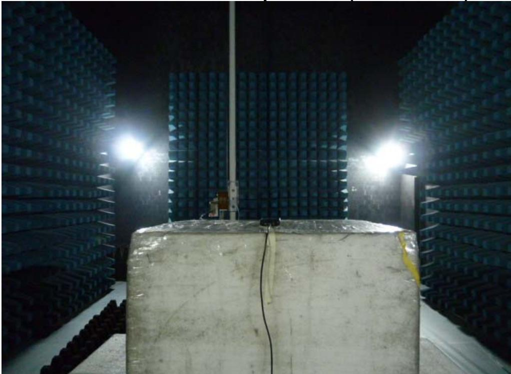
**Radiated Emission Set up Photos (Front View)**
