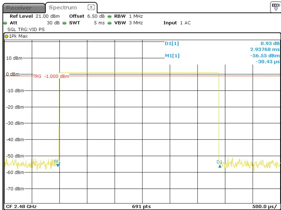
**EDR ( $\pi/4$ -DQPSK):****Pulse time, Low Channel, 2DH1**
