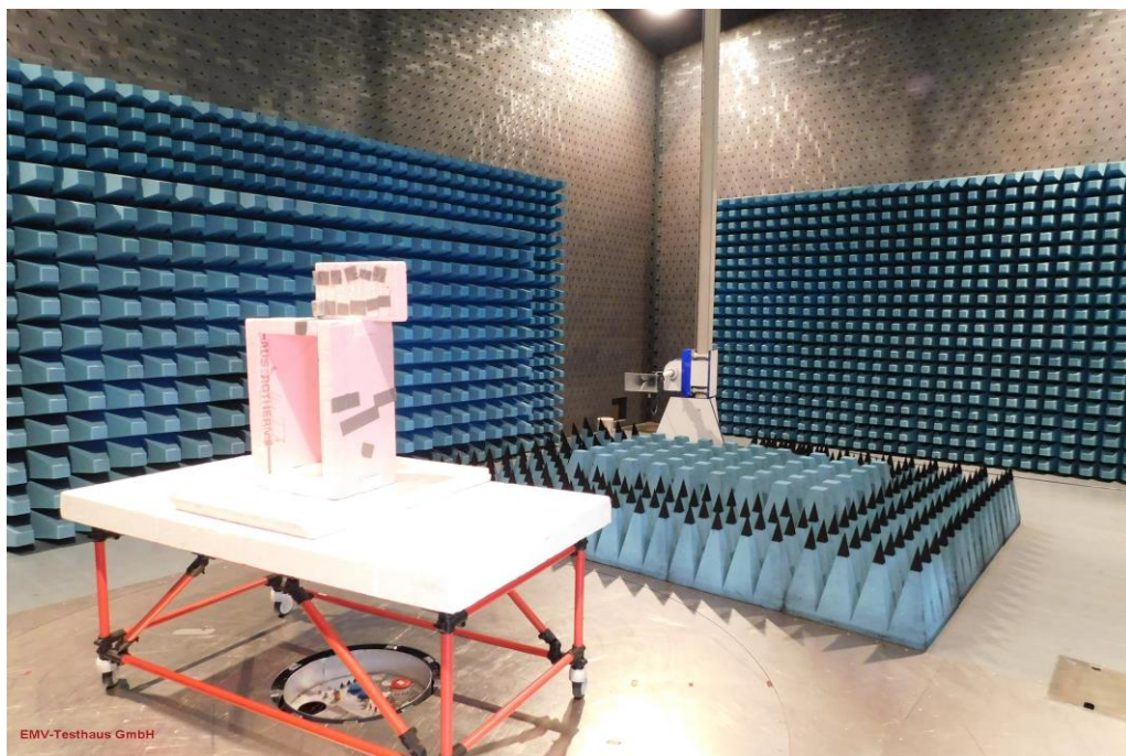
Picture 5: SAC, radiated emission 1 GHz – 10 GHz (front view)
