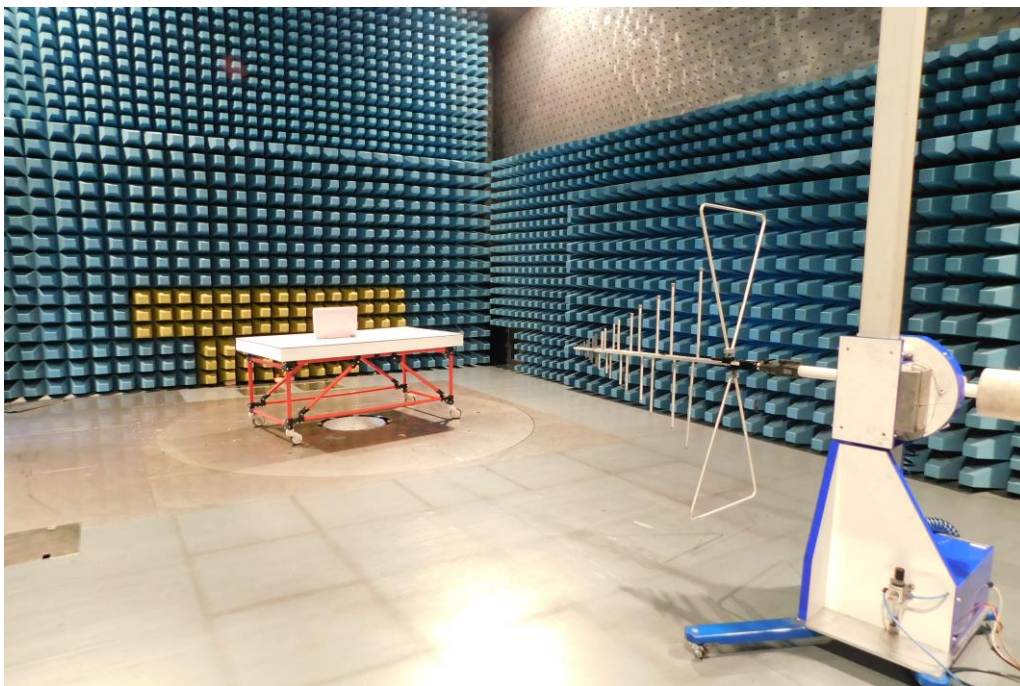
Picture 4: SAC, radiated emission test 30 MHz -1 GHz (rear view)
