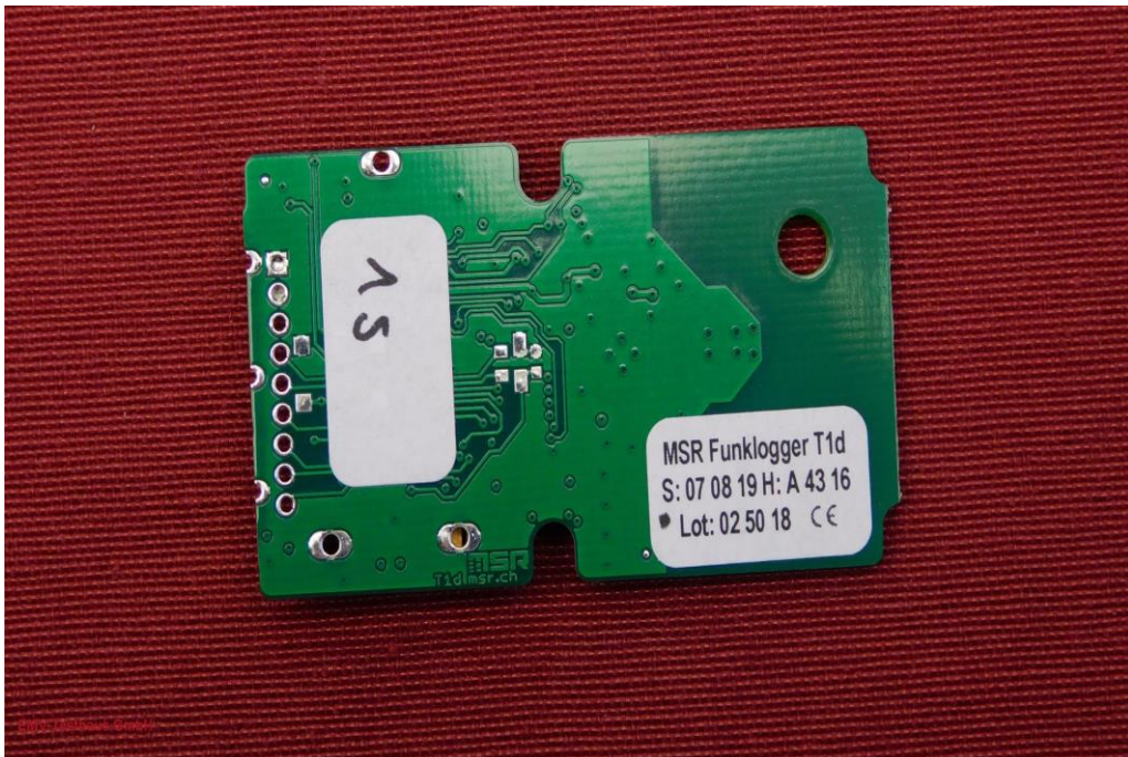
Picture 2: Transmitter without cover - top view
