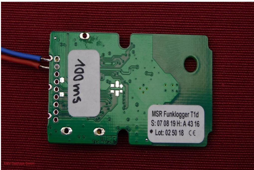
Picture 8: Transmitter without cover - bottom side
