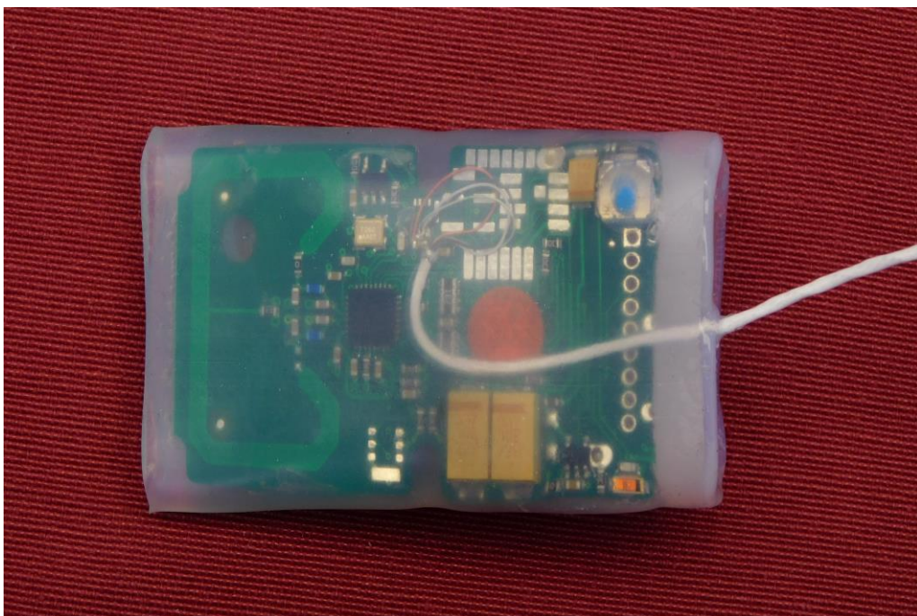
Picture 2: Transmitter with plastic cover- bottom side
