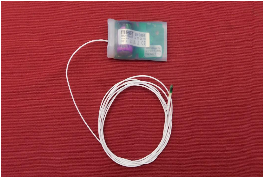
Picture 3: Transmitter with plastic cover and sensor - top side
