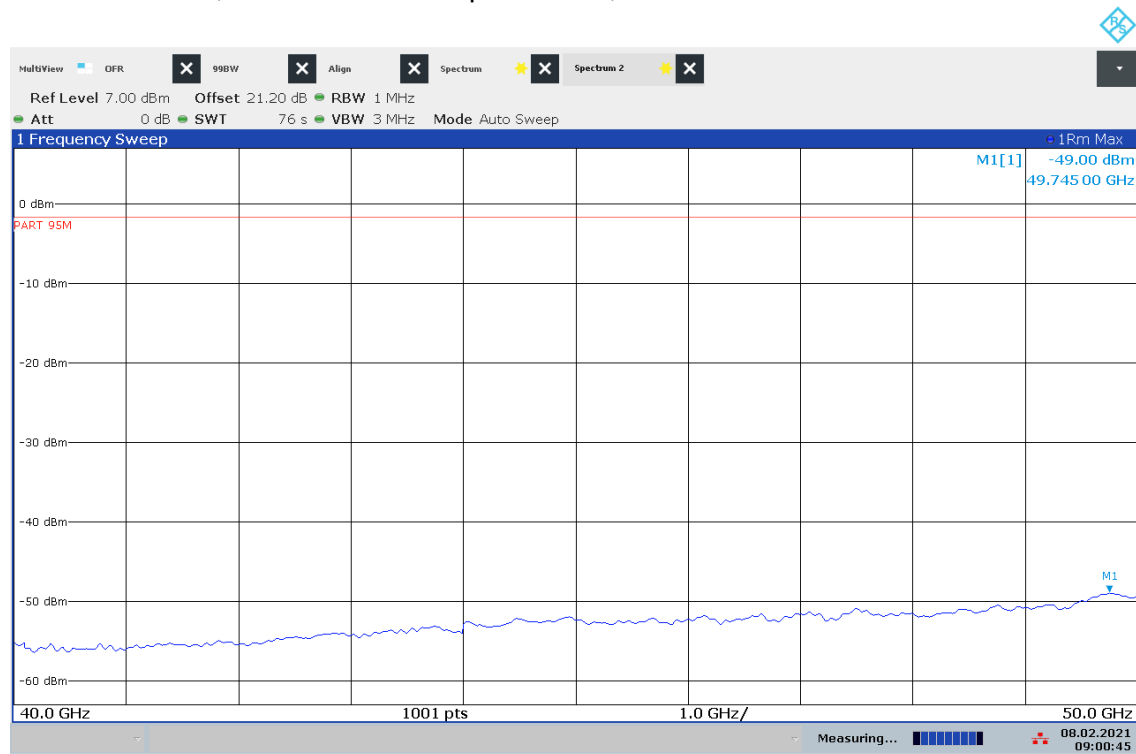
Plot 28: 40 GHz – 50 GHz, vertical / horizontal polarization, Mode 3
