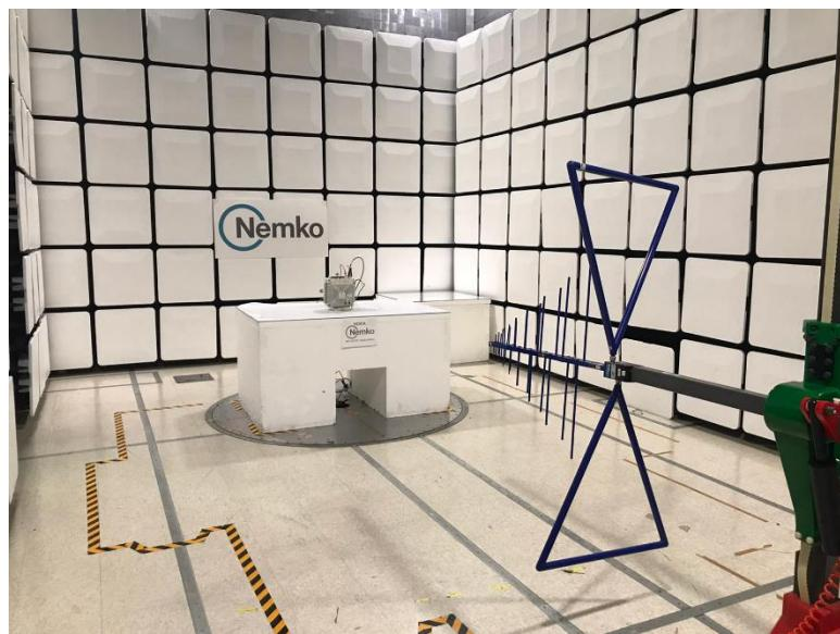
**Radiated tests – above 1GHz**
