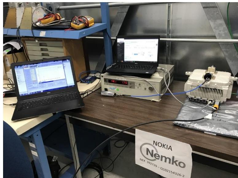
**Radiated tests – below 1GHz**
