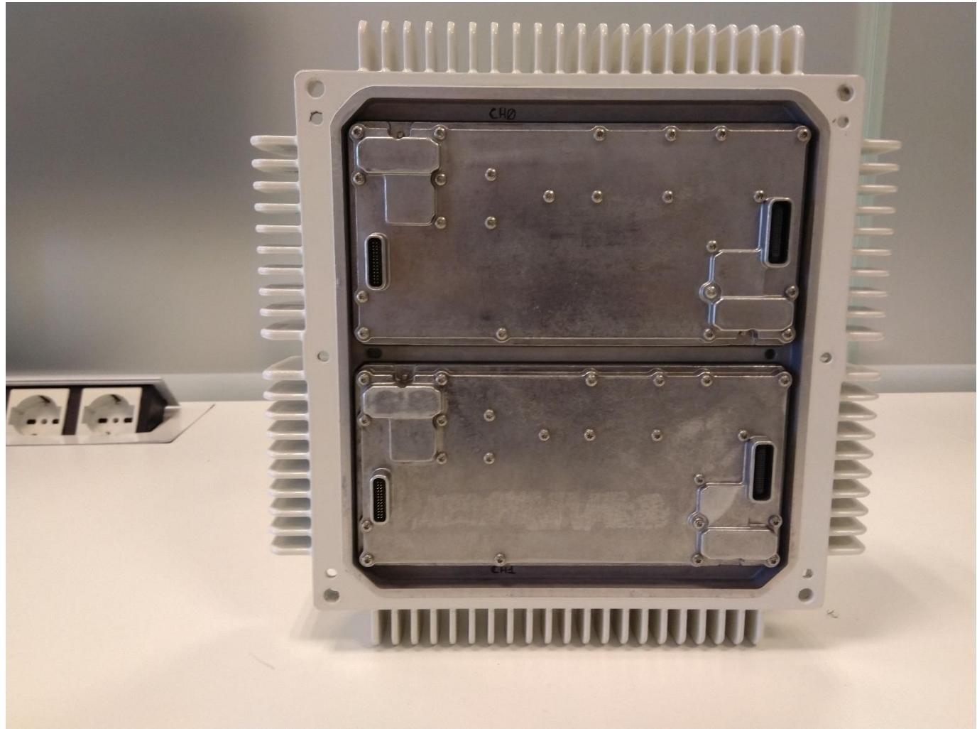
1.6 RF Assemblies with the RF Cover for Twin and RF PBAs, without the RF Shields.
