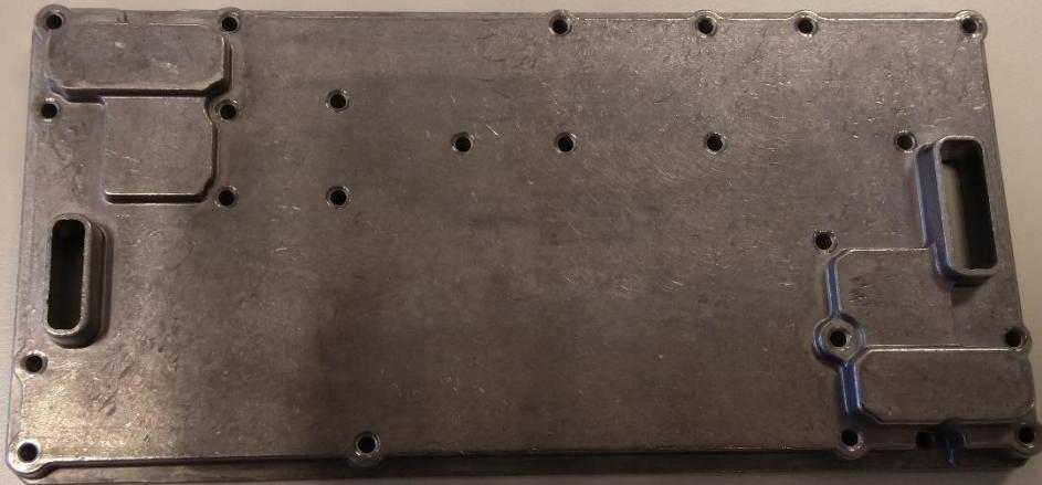
1.11 RF Shield Internal View, 1 of 2 ea, Twin Boards.
