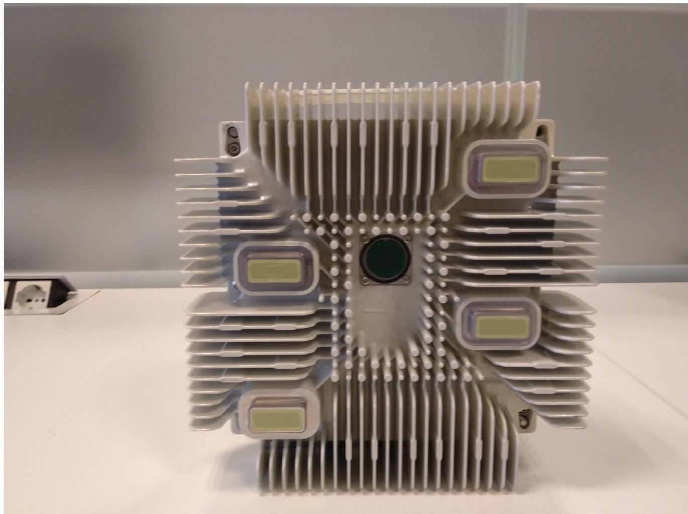
1.3 Antenna Interface Module Twin Diplexer (AIM-T-D), Antenna mounting surface
