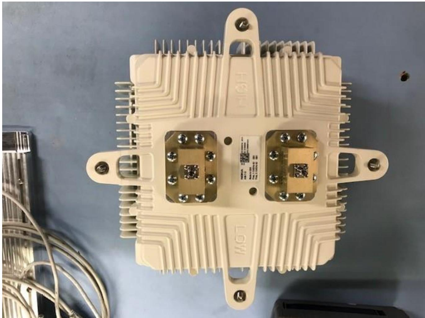
1.4 Antenna Interface Module Twin Diplexer (AIM-T-D), radio mount view.
