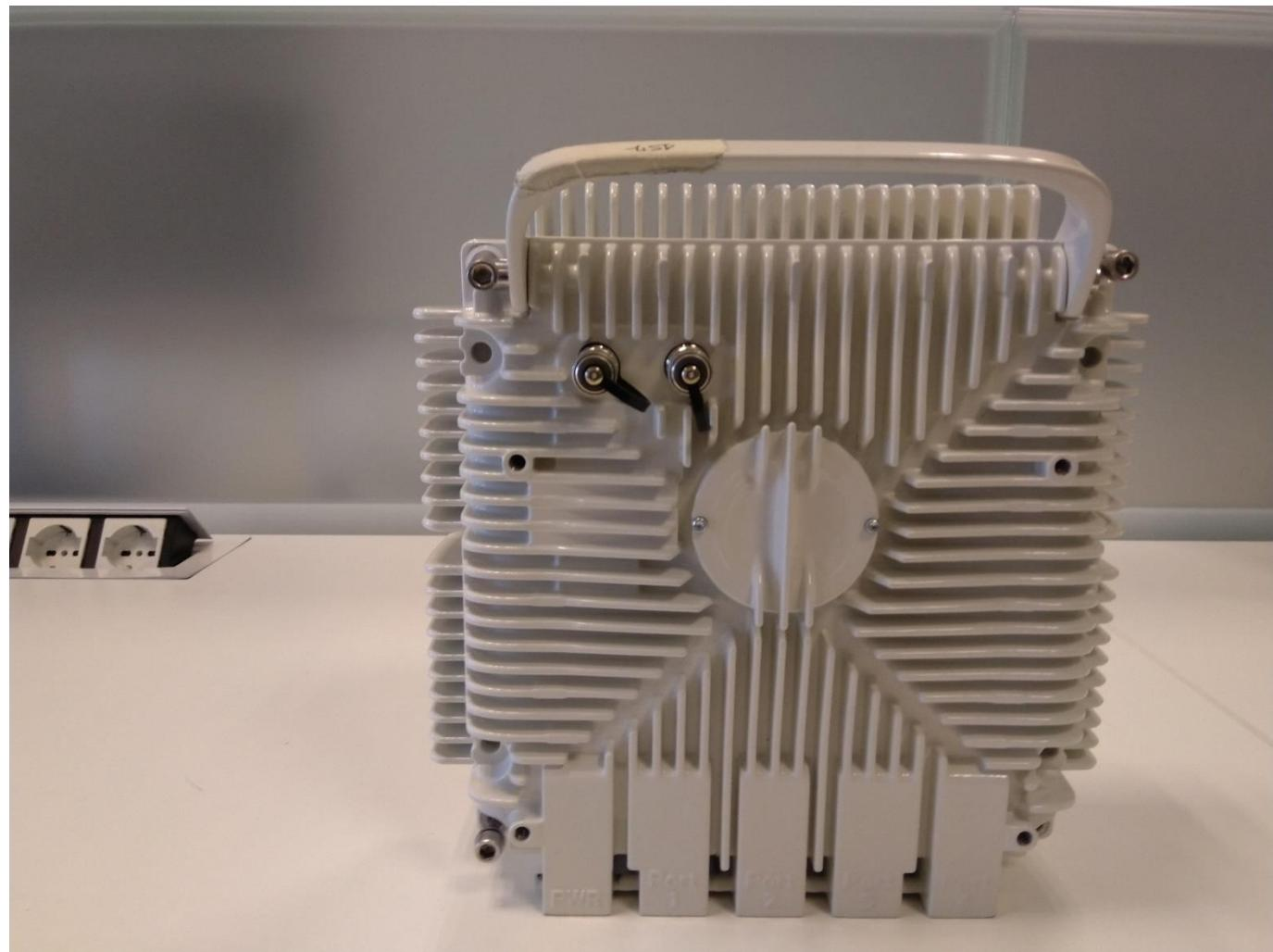
1.2 UBT-T Rear View without Antenna Interface Module (AIM-T-D)
