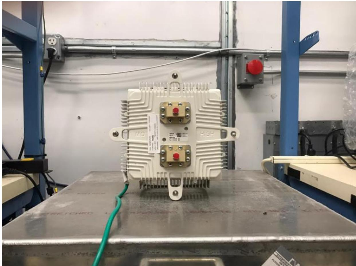
1.7 UBT-T Side view with Antenna Interface Module (AIM-T-D)
