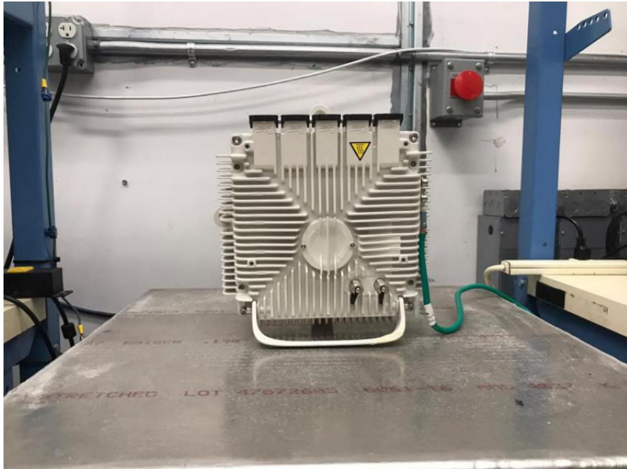
1.6 UBT-T Rear view with Antenna Interface Module (AIM-T-D)
