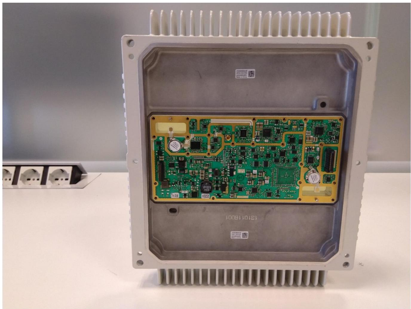
1.7 RF Cover without RF PBA and without RF Shield.
