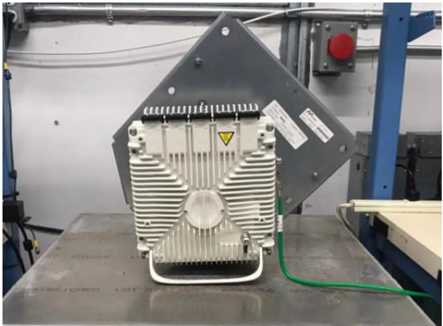
1.6 UBT-S Rear view with Antenna Interface Module Single (AIM-S) attached to an antenna mount for test.
