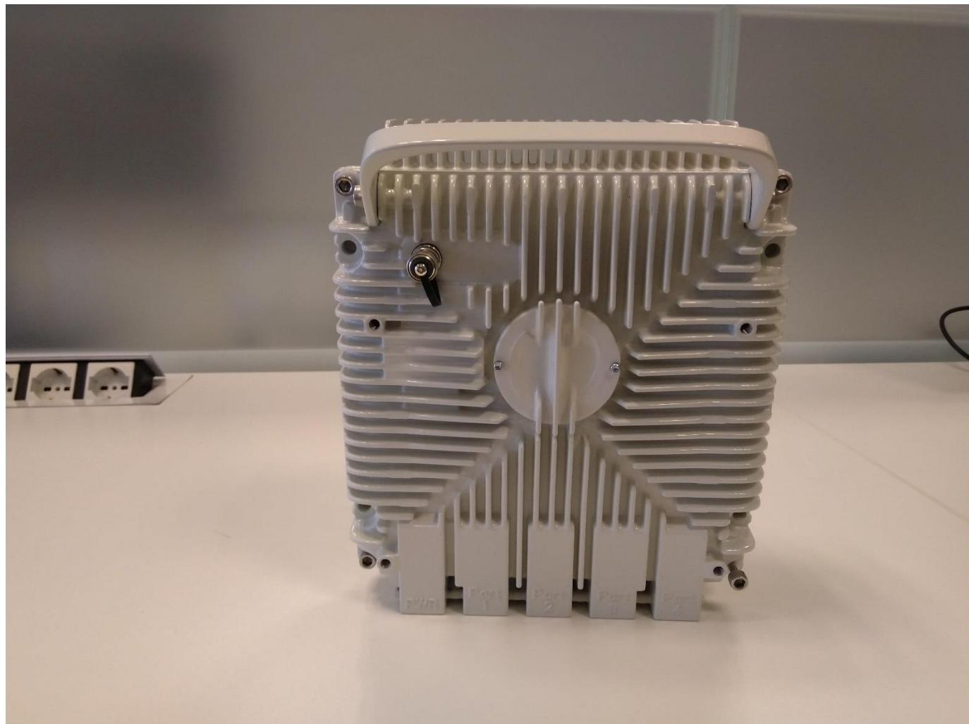
1.2 UBT-S Rear view without Antenna Interface Module Single (AIM-S)
