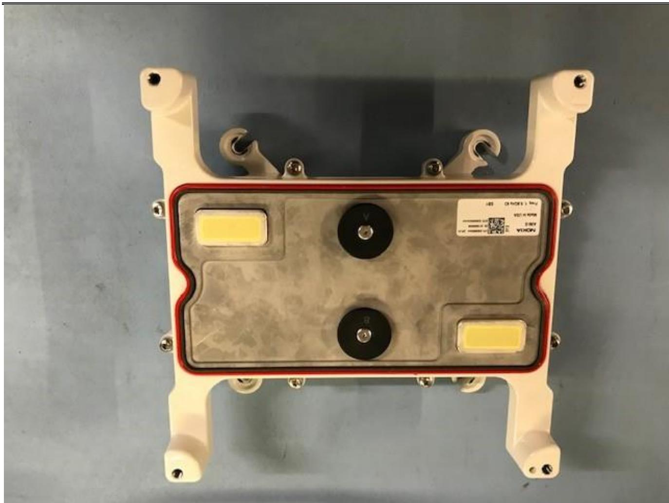
1.5 UBT-S Top general view with Antenna Interface Module Single (AIM-S) attached to an antenna mount for test.
