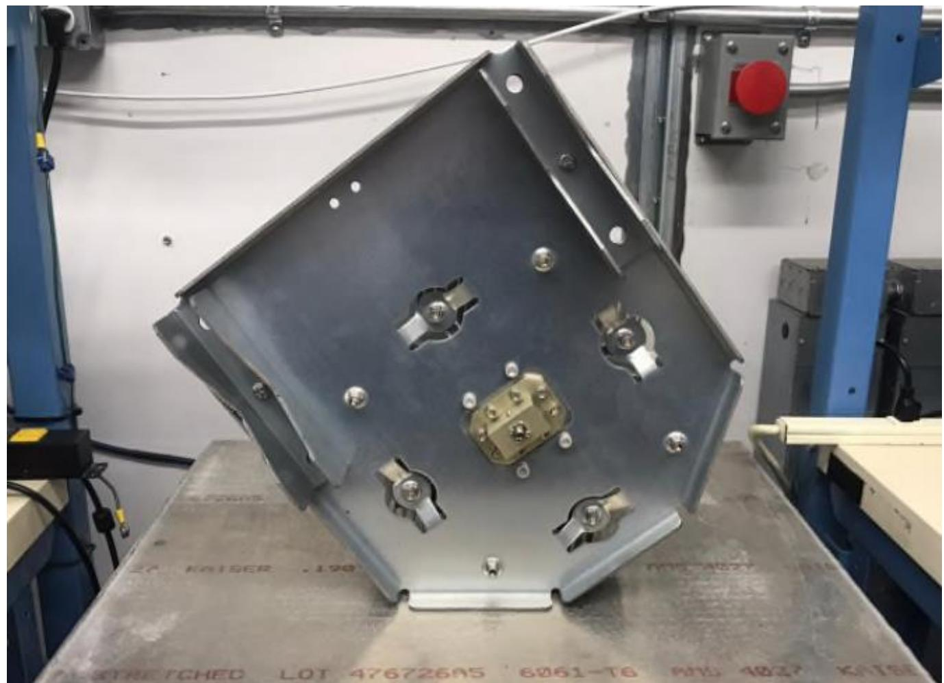
1.7 UBT-S Side view with Antenna Interface Module Single (AIM-S) attached to an antenna mount for test.
