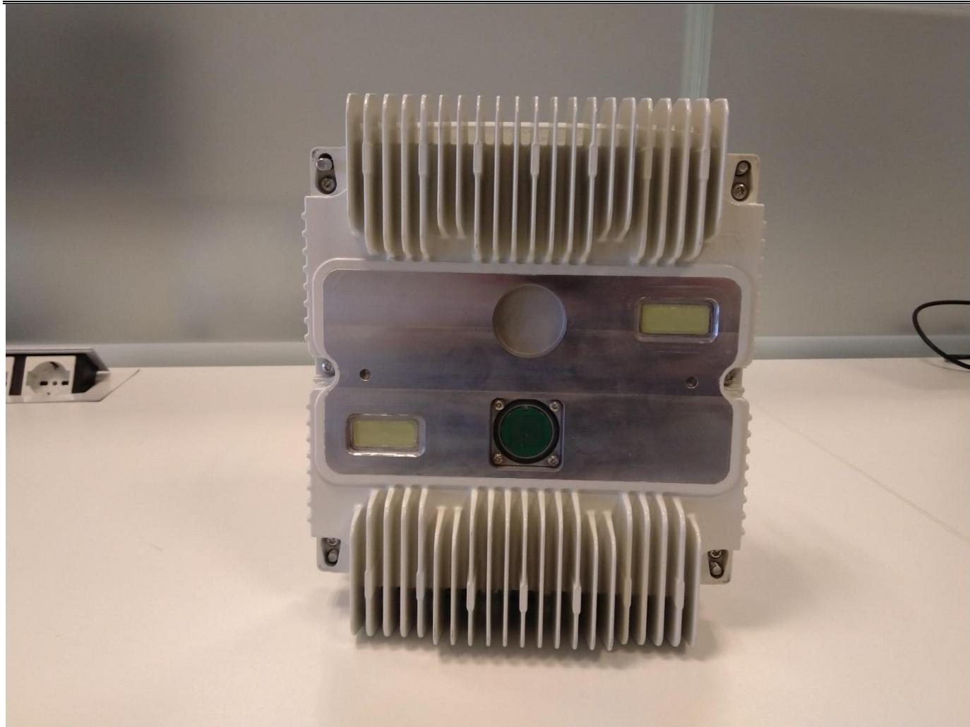
1.3 Antenna Interface Module Single – Antenna Mounting side
