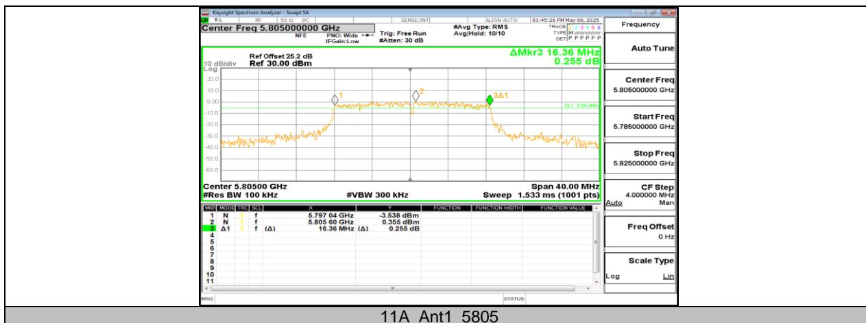
**10.4. APPENDIX D: MAXIMUM CONDUCTED OUTPUT POWER****10.4.1. Test Result**
