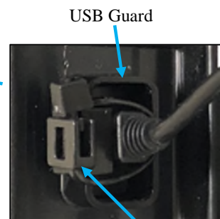
Figure 5c: STA-STRAP (item 4) Secure to USB guard
