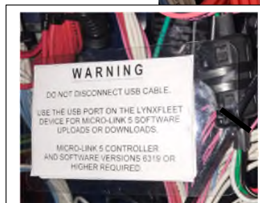
Figure 5d: Add new warning tag and label (item 7 and 6) here on the USB harness.
