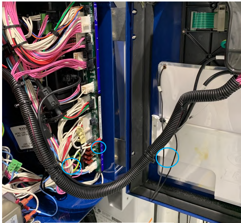
Figure 7a: Securing wire harness
