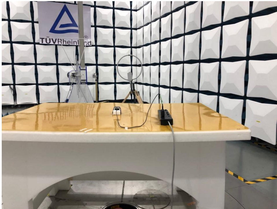
Photograph 1: Set-up photo for Radiated Spurious Emission, 9KHz - 30MHz
