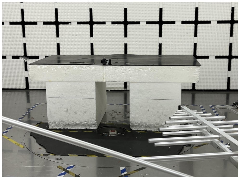
Radiation Emission Test Setup (30MHz to 1GHz)
