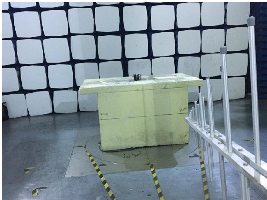
Radiation Emission Test Setup (30MHz to 1GHz)
