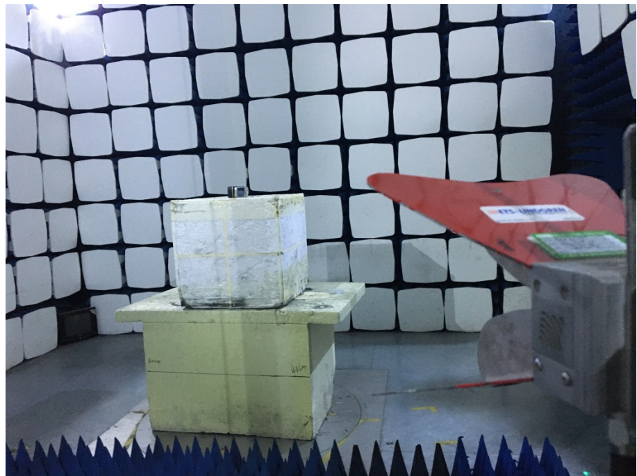
Radiation Emission Test Setup (1GHz to 18GHz)
