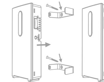
To dismount the chime, push it inward to the installation mount and slide it downward as shown below.
