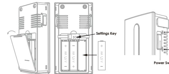
Enter the smart door lock into pairing mode. (Refer to the manual of the smart door lock on how to enter pairing mode.) Briefly press the settings key at the back of the chime twice (2x). The chime enters the pairing mode. The red and white LED indicators flash alternately and slowly. If pairing is successful, the white LED will be ON for 2S. The red LED will be ON for 2S if the pairing fails or timeout in 30s.
