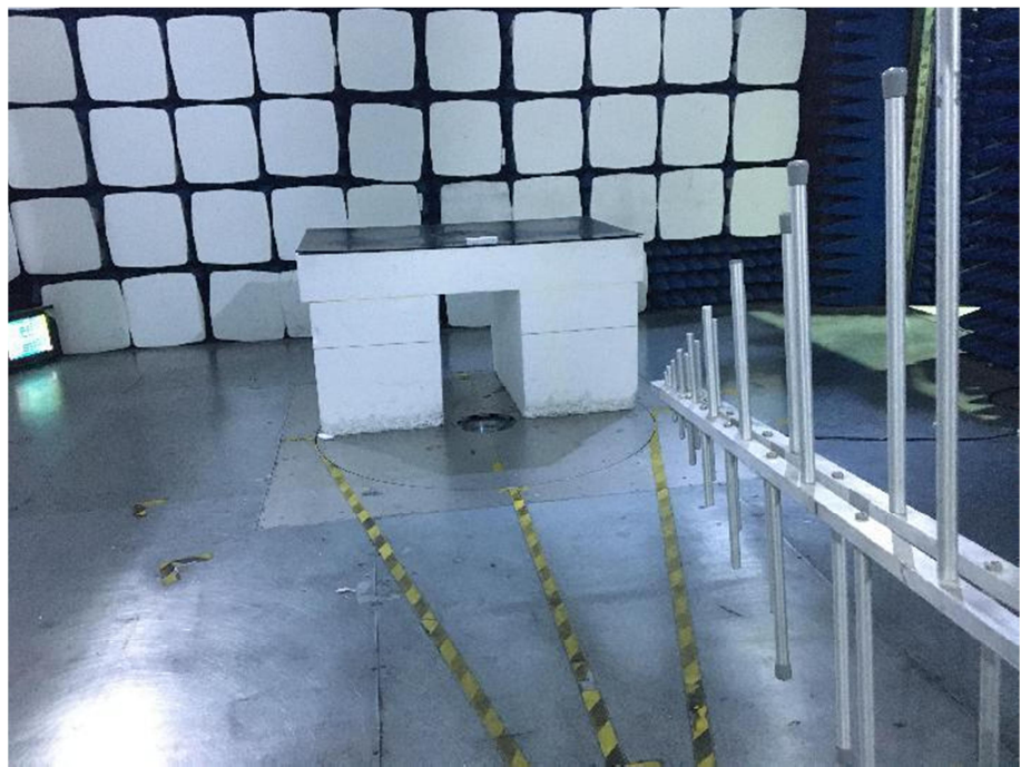
Radiation Emission Test Setup (30MHz to 1GHz)
