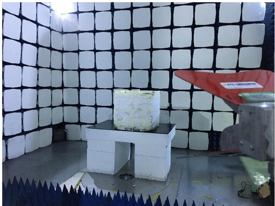
Radiation Emission Test Setup (1GHz to 18GHz)
