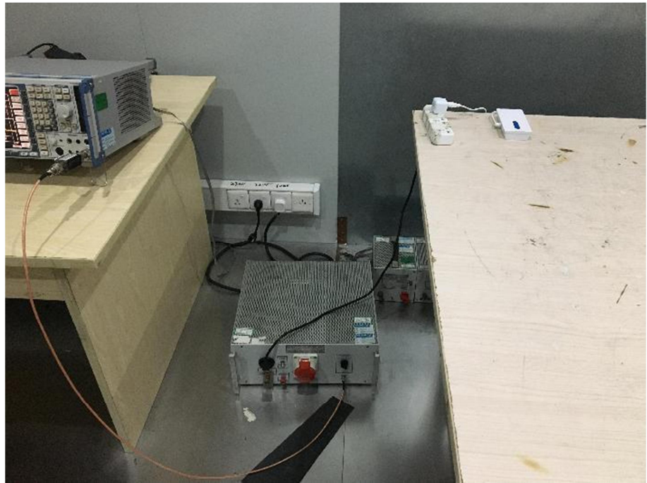
Conducted Emission Test Setup
