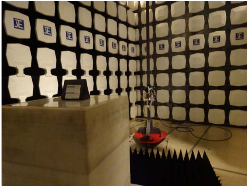
Measurement of Radiated Emission Test Set Up
