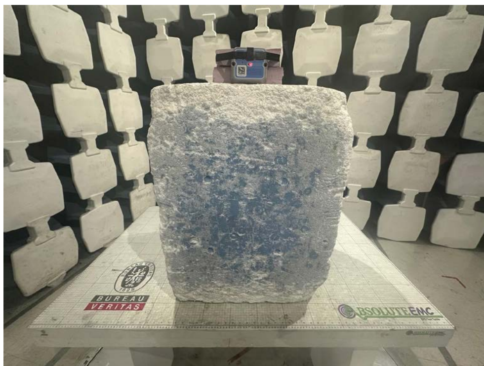
EUT Setup for radiated emissions
