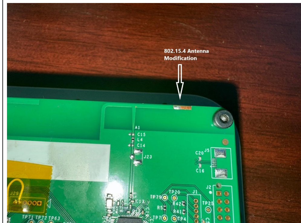
Antenna modification closeup
