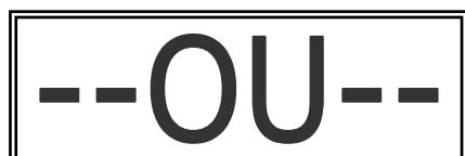
Show overloading. If there is no weight on scale body, no overloaded, the down-lead from load cell to transmitter is wrong linked or cut.
