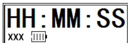
Display Time, serial number and battery power. Or no signal, please check the Antenna or battery.
