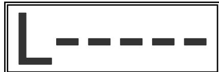
After turning on power, if hand-held instrument displays above, shows batteries of hoist scale end under-voltage, please recharge. After several seconds transmitter of hoist scale shutdown automatically.
