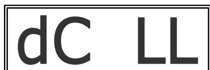
After power-on self-test, displays above and light up under-voltage sign, after two seconds shutdown automatically. Shows hand-held instrument batteries under-voltage, cannot be used normally, please recharge.
