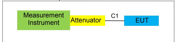
For Peak-to Average Ratio, Occupied Bandwidth, Conducted Band edge and Conducted Spurious Emission
