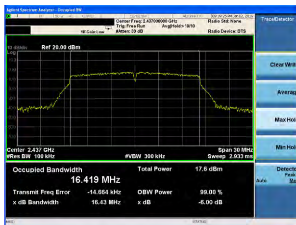
(802.11g) 6dB Bandwidth plot on channel 6
