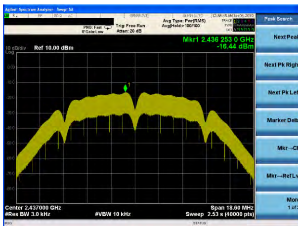
(802.11b) PSD plot on channel 6
