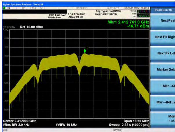
(802.11b) PSD plot on channel 6
