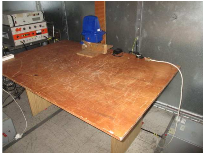
Figure 1. Conducted Emission AC Line Test
