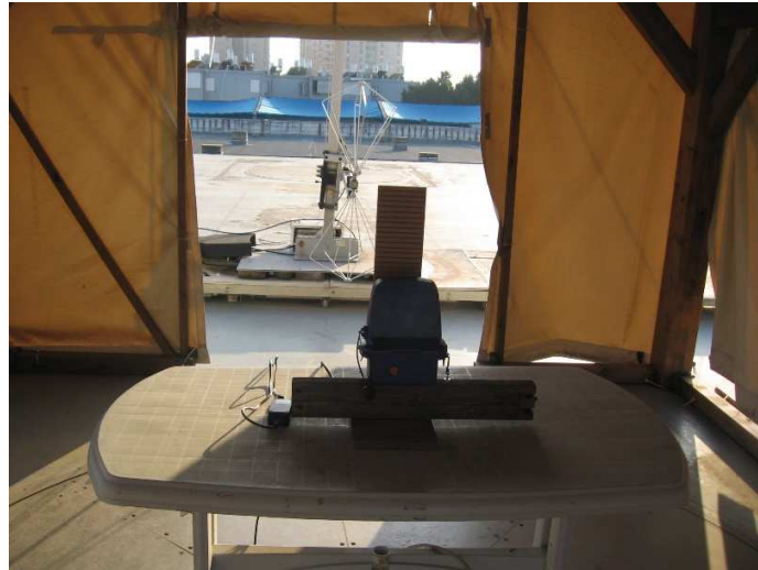
Figure 3. Radiated Emission Test, 30.0-200.0MHz
