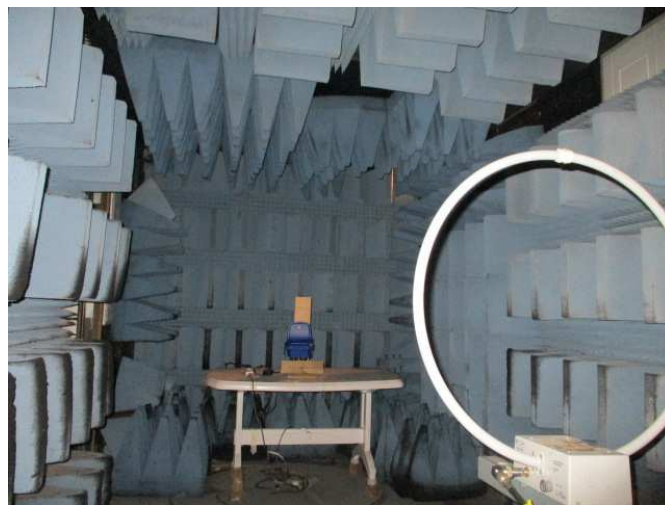
Figure 2. Radiated Emission Test, 0.009 30.0MHz
