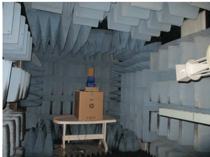
Figure 6. Radiated Emission Test, 18-26.5GHz
