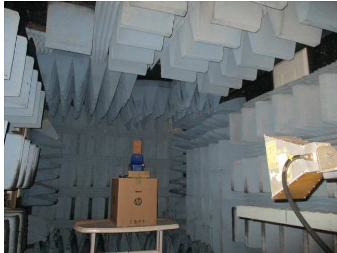
Figure 5. Radiated Emission Test, 1.0-18.0GHz
