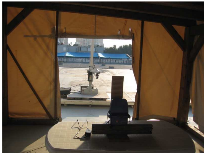
Figure 4. Radiated Emission Test, 200.0-1000.0MHz
