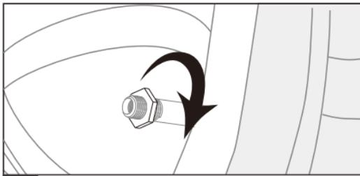
1 Rotate the nut onto vehicle tire valve.
