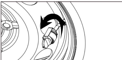
3 By enclosed spanner rotate the nut anti-clockwise until it's pressing against sensor.
