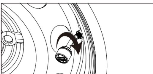
2 Mount sensor on valve clockwise, screw down to bottom and tight.
