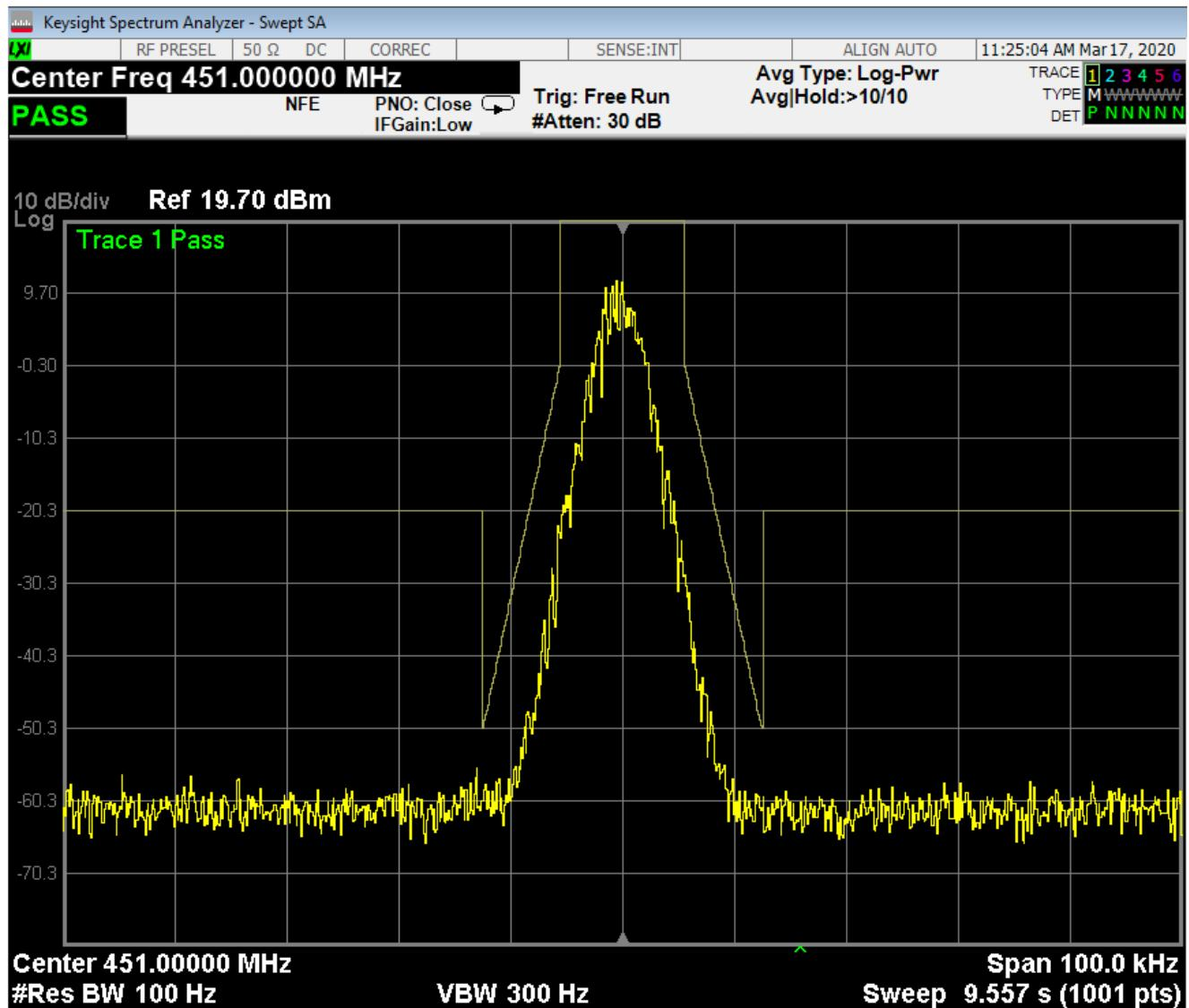
451.000 MHz, 25.0 kHz spacing, FSK 512
