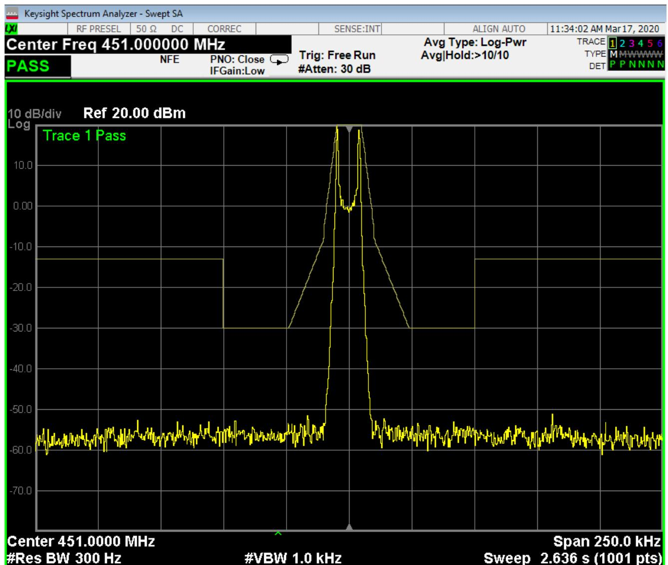
451.000 MHz, 25.0 kHz spacing, FSK 1200
