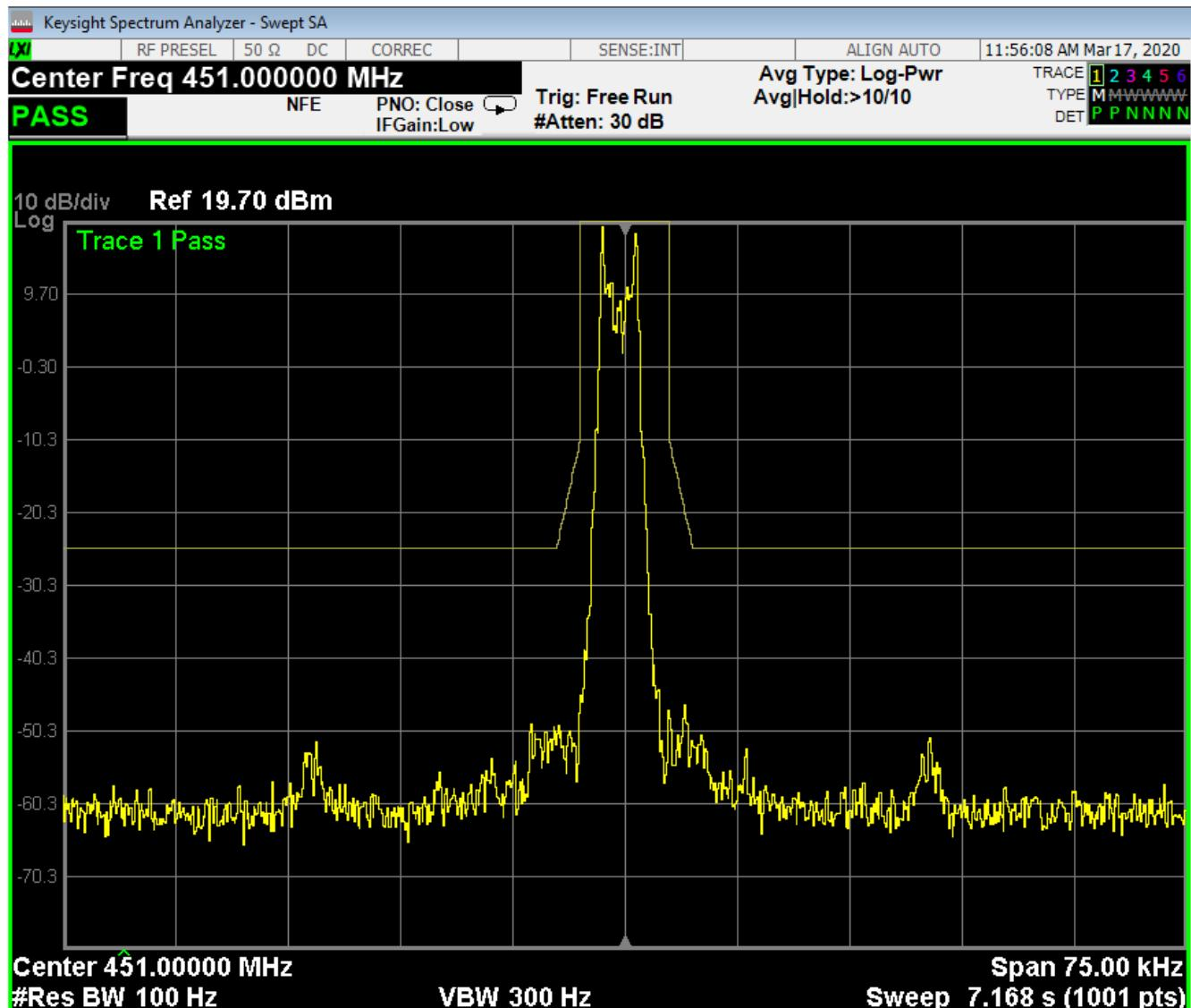
421.000 MHz, 6.25 kHz spacing, GFSK 4800
