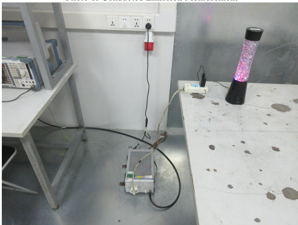
Photo of Conducted Emission Measurement
