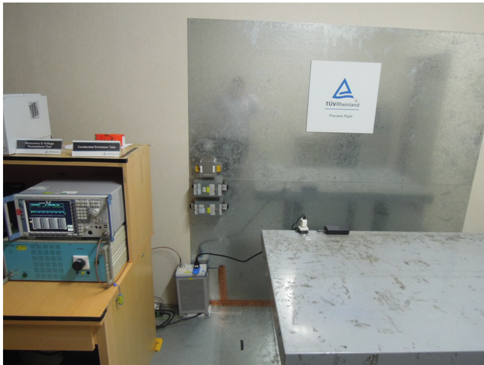
Photograph 17: Set-up for Mains Conducted testing (Front View)
