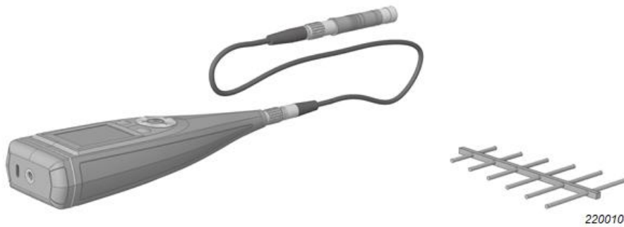
Fig. 3.5 The direction for the least immunity to magnetic power-frequency fields
