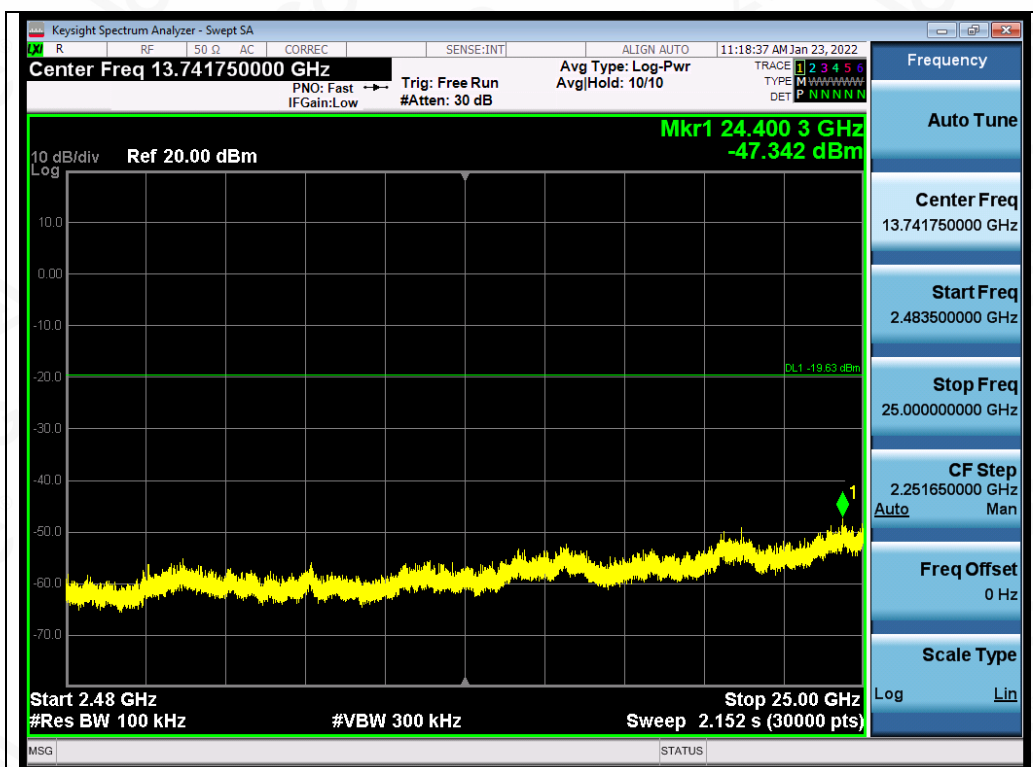
Test_Graph_LE1M_ANT1_2402_1Mbps_Higher Band Emissions
