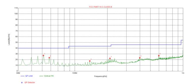
Suspected List Freq. Factor Reading Level Limit Margin Height Angle NO. Polarity [dB] [dB] [dBµV/m]  $[dB\mu V/m]$  $[dB\mu V/m]$ [MHz] [cm] [°] 51.3614 -13.86 41.10 27.24 40.00 12.76 100 78 Vertical 1 2 58.1582 -14.88 38.24 23.36 40.00 16.64 100 87 Vertical 137.7778 -19.04 17.65 43.50 25.85 348 Vertical 3 36.69 100 -14.76 22.25 4 211.5716 37.01 43.50 21.25 100 121 Vertical 5 398.9690 -10.43 33.62 23.19 46.00 22.81 100 Vertical
