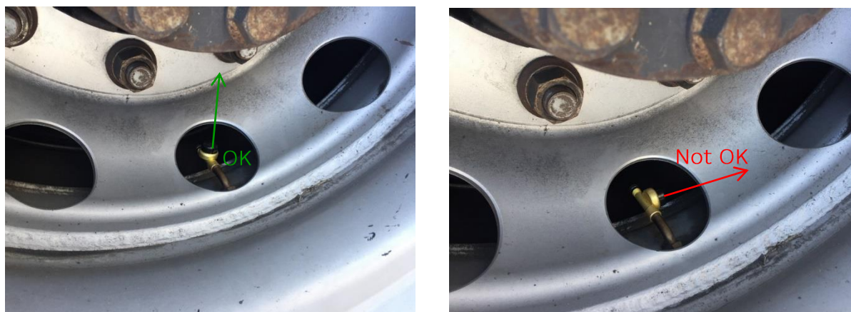
Fig. 3 - Examples of sensor orientation with high (left) and low (right) signal strength
