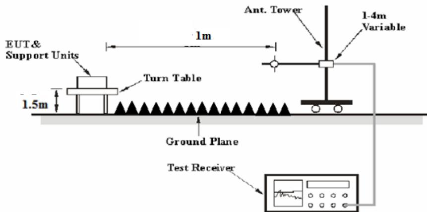
The radiated emission Below 1GHz tests were performed in the 3 meters chamber test site A , above 1GHz tests were performed in the 3 meters chamber test site B, using the setup accordance with the ANSI C63.10-2013. The specification used was the FCC 15.209, and FCC 15.407 limits and RSS-247, RSS-Gen limits.
