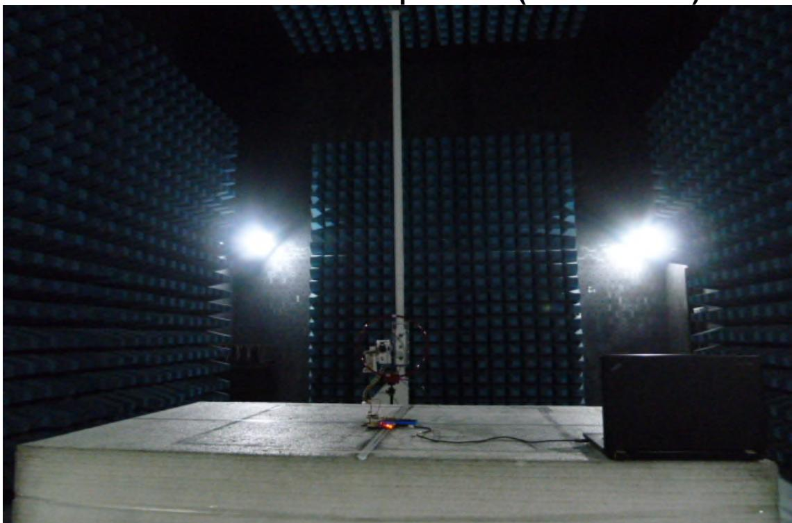
**Radiated Emission Set up Photos (Below 1GHz)**
