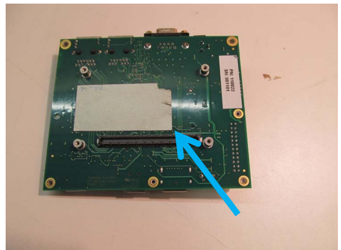
Shielding material at Connector Board
