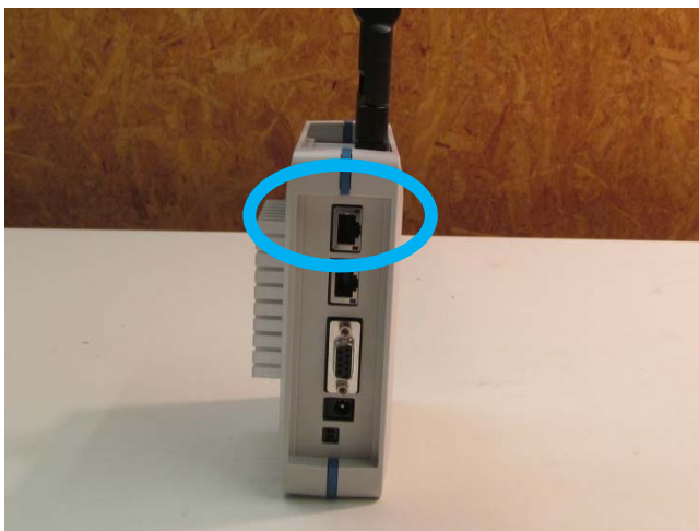
Deactivated Ethernet Port
