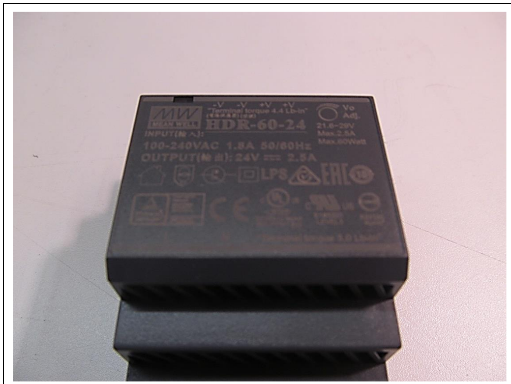
Photograph A4-6: Label of DIN Rail AC/DC adaptor (supply for ancillary current loop sensor)
