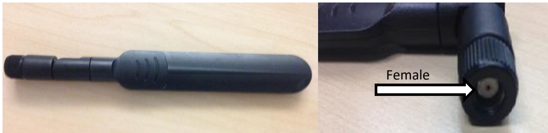
Figure 19: Wi-Fi "Rowing Stick" antenna with RP-SMA female connector
