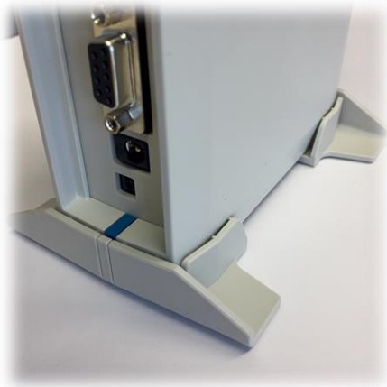
Figure 2: Desk placement of the MYNXG EDGE FCR 3
