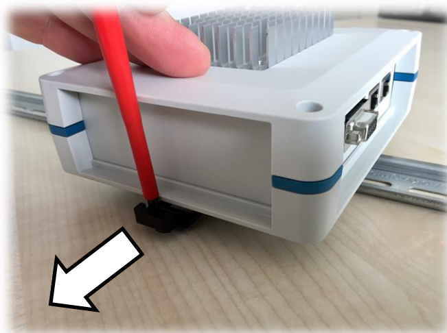
Figure 15: Releasing the DIN-rail fixture
