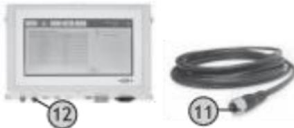
Connect one of the plugs (11) of the connection cable to one of the two M12 sockets (12) on the Master and screw on the knurled coupling nut. Both connections of the Master can be used at the same time.
