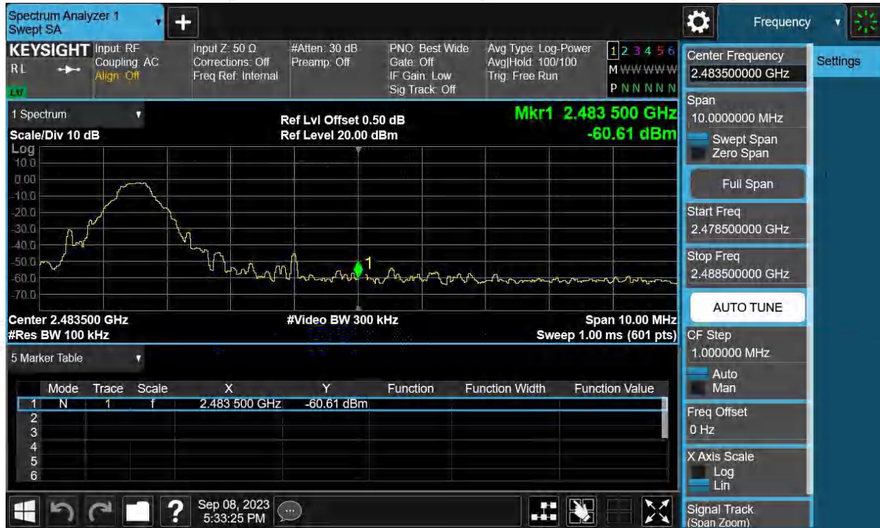
Figure 45: The plots of Conducted Spurious Emission & Authorized-band band-edge, 2480MHz, BLE-2Mbps, Conducted spurious emissions 30MHz-3GHz
