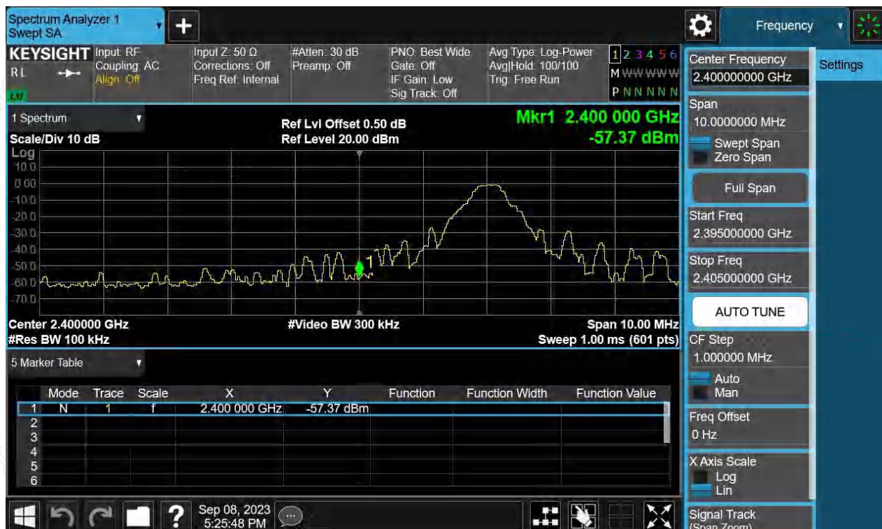
Figure 26: The plots of Conducted Spurious Emission & Authorized-band band-edge, 2402MHz, BLE-1Mbps, Band Edge
