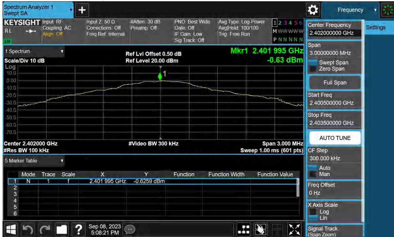
Figure 37: The plots of Conducted Spurious Emission & Authorized-band band-edge, 2402MHz, BLE-2Mbps, Band Edge
