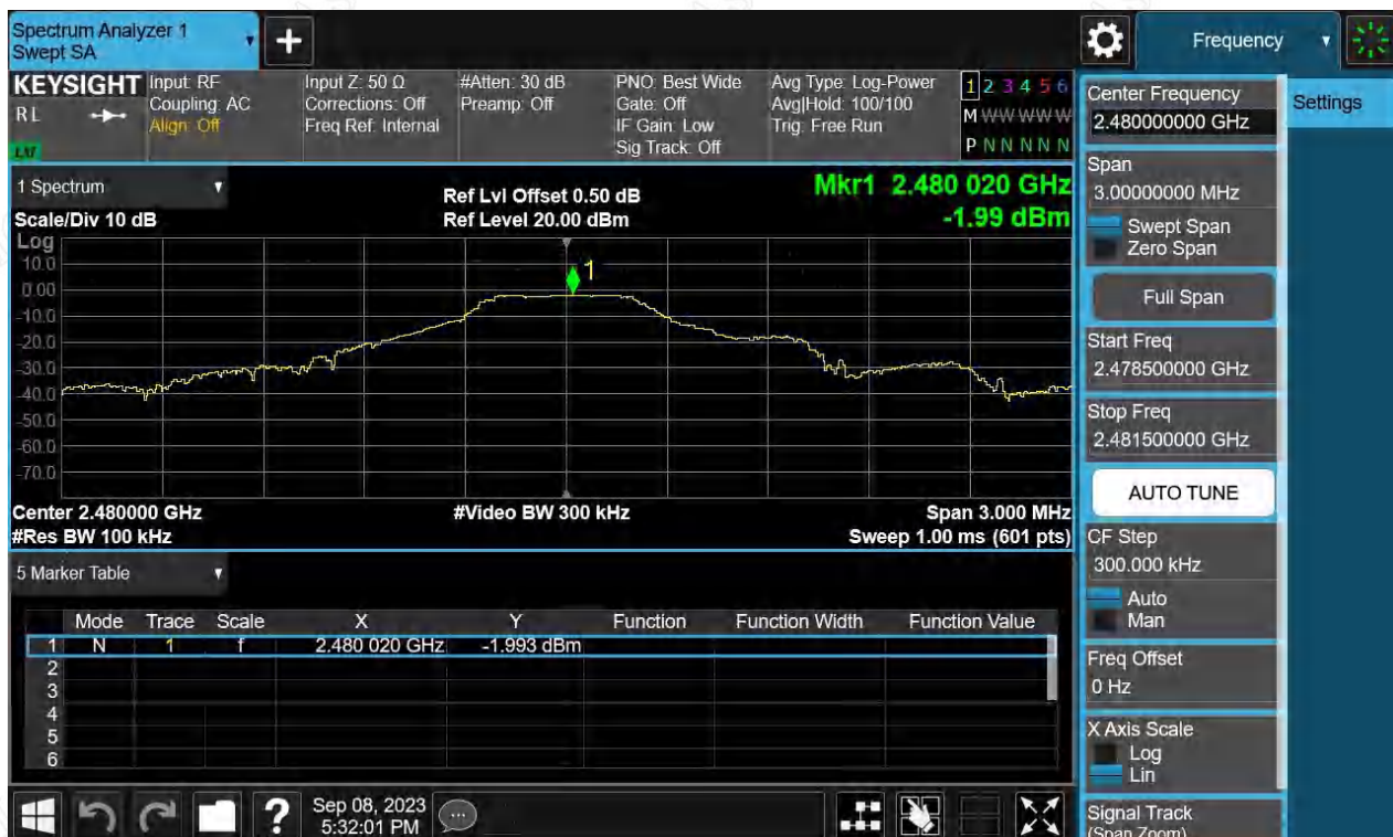
Figure 32: The plots of Conducted Spurious Emission & Authorized-band band-edge, 2480MHz, BLE-1Mbps, Carrier Level
