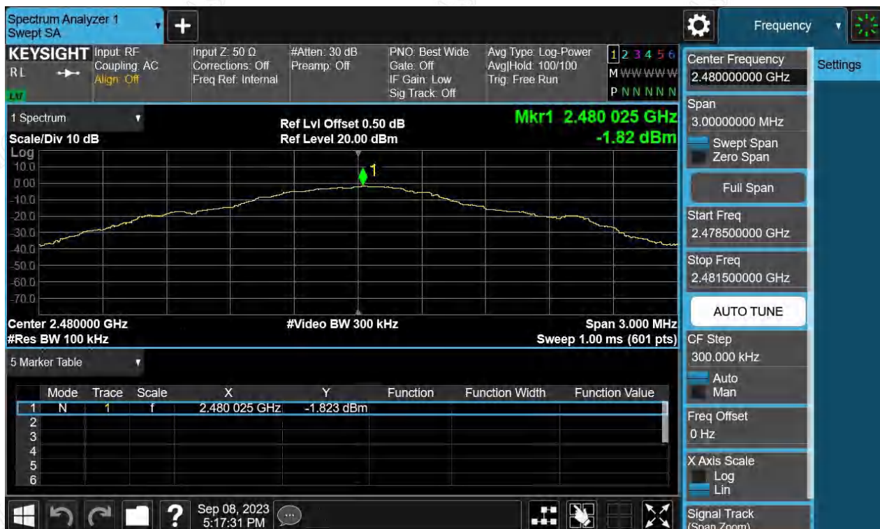
Figure 43: The plots of Conducted Spurious Emission & Authorized-band band-edge, 2480MHz, BLE-2Mbps, Carrier Level
