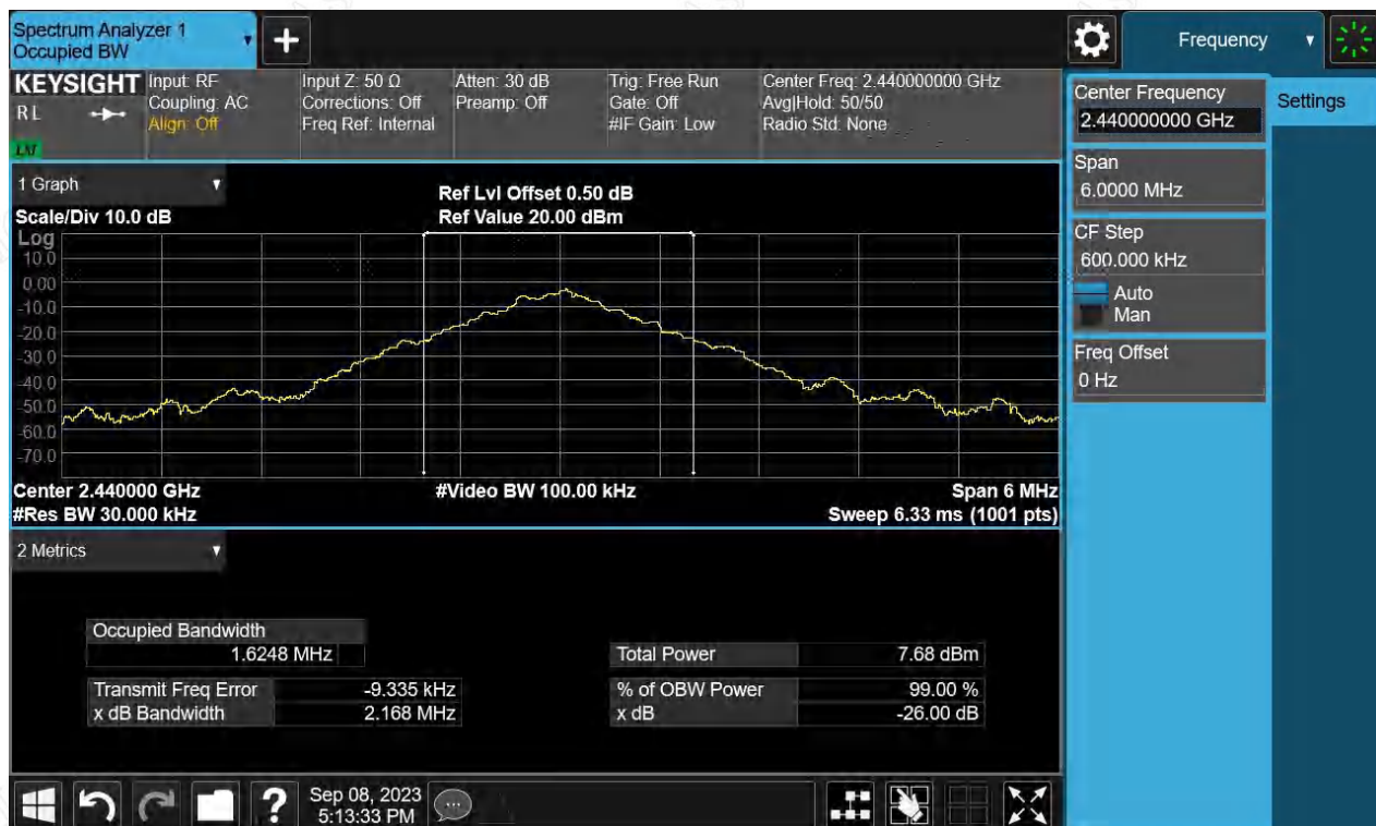
Figure 16: The plots of 99% Bandwidth, BLE-2Mbps, 2440MHz
