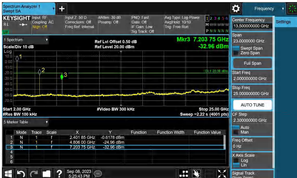
Figure 28: The plots of Conducted Spurious Emission & Authorized-band band-edge, 2402MHz, BLE-1Mbps, Conducted spurious emissions 2GHz-25GHz
