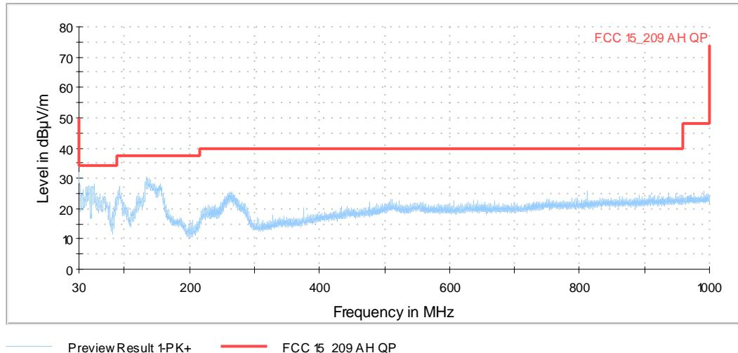
The following frequencies were identified during the preliminary measurement, a final measurement on the OATS will be carried out.
