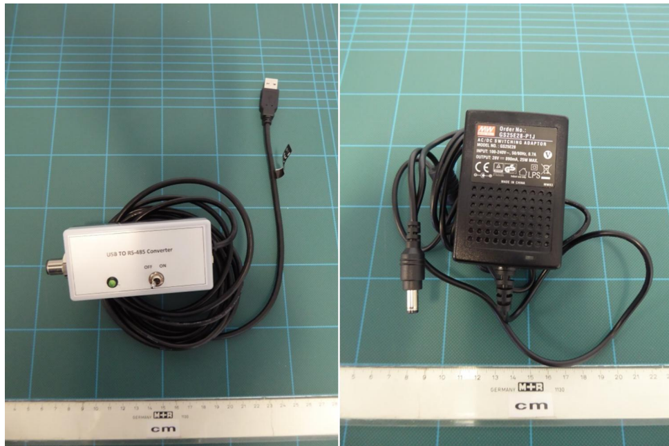
Ancillary equipment - USB to RS485 converter and power supply
