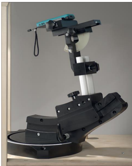
F-2. Device Holder for Transmitters
