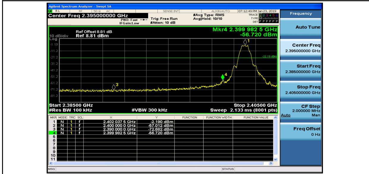
Band-edge for RF Conducted Emissions\_BLE\_2480\_Hopping Off
