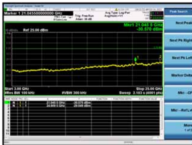
GFSK MIDDLE CHANNEL, SPURIOUS 3 GHz ~ 25 GHz
