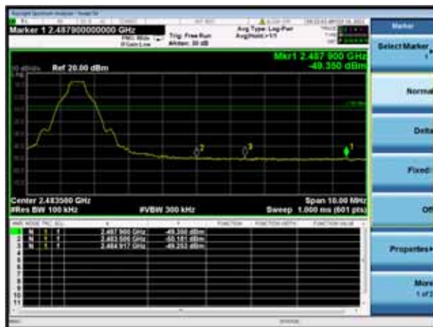
GFSK HIGH CHANNEL, BAND EDGE
