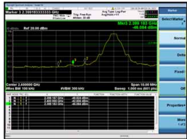
GFSK LOW CHANNEL, BAND EDGE
