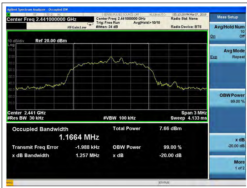
(8-DPSK, Channel 39, 2441MHz)
