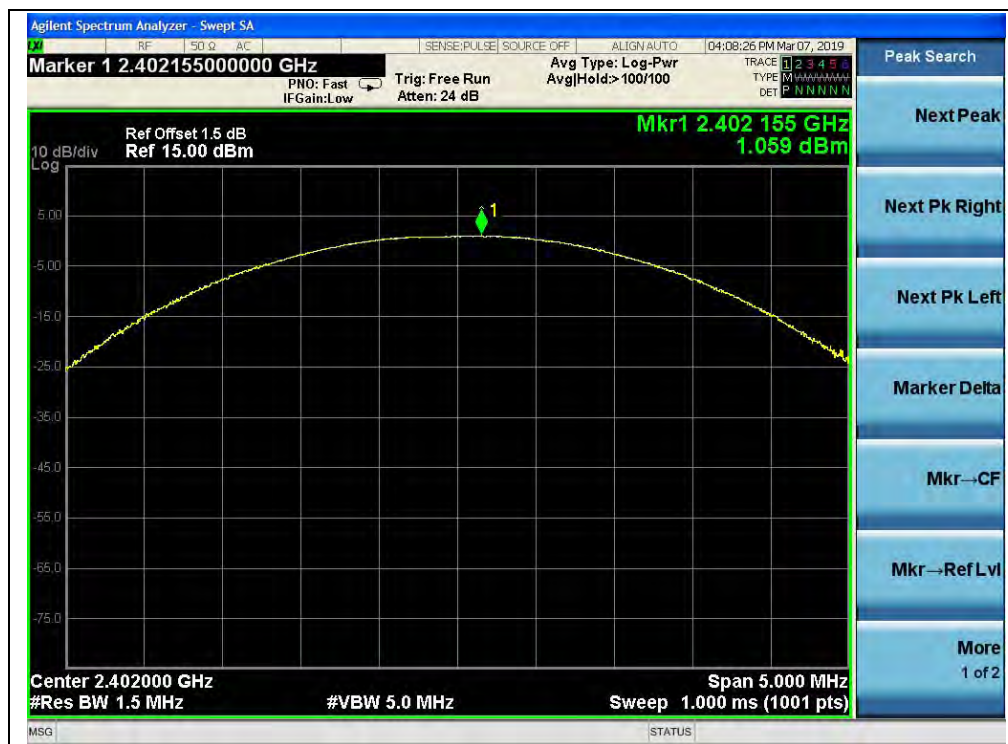
(π/4-DQPSK, Channel 0, 2402MHz)
