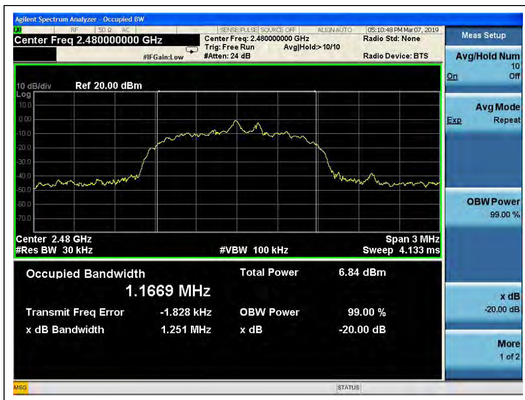
(8-DPSK, Channel 78, 2480MHz)
