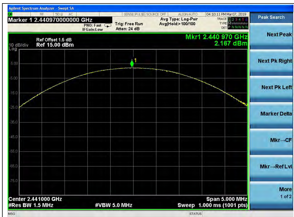
(8-DPSK, Channel 39, 2441MHz)
