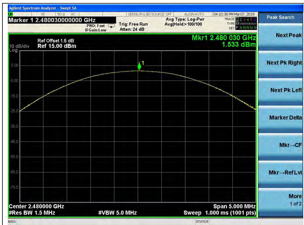
(8-DPSK, Channel 78, 2480MHz)
