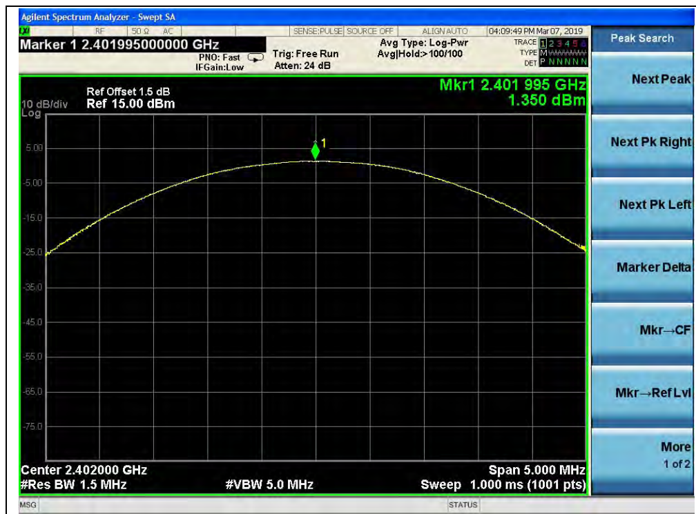
(8-DPSK, Channel 0, 2402MHz)
