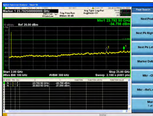
GFSK (BLE 1Mbps) MIDDLE CHANNEL, SPURIOUS 2 GHz ~ 25 GHz
