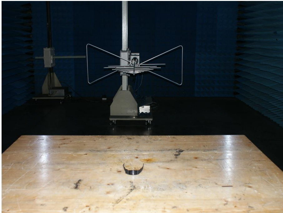
Photograph 3: Set-up for Radiated Spurious Emission, 30MHz - 1GHz
