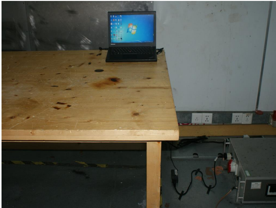
Photograph 1: Set-up for Conducted Emission on AC Mains
