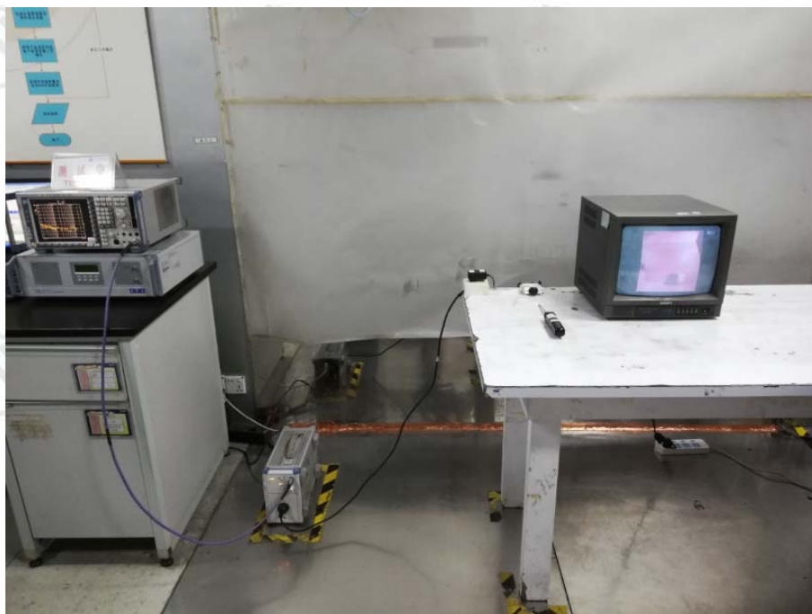
CONDUCTED EMISSION TEST SETUP
